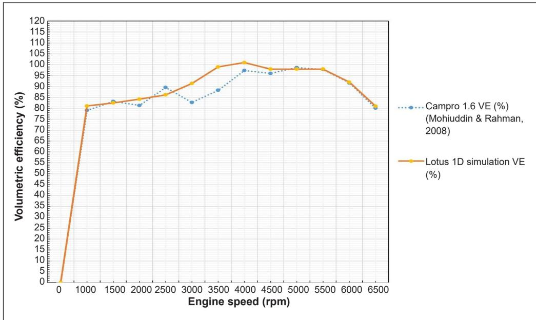
Figure 2. Volumetric efficiency comparison between experimental (Mohiuddin & Rahman, 2008) and Lotus 1D simulation across a range of rpm
