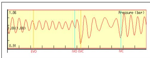
Figure 5. Pressure fluctuation at intake port for full engine cycle at 1000 rpm
