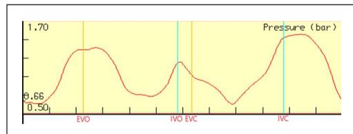
Figure 6. Pressure fluctuation at intake port for full engine cycle at 7000 rpm
