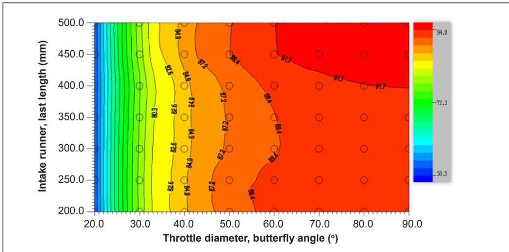
Figure 8. Volumetric efficiency at 3000 rpm
