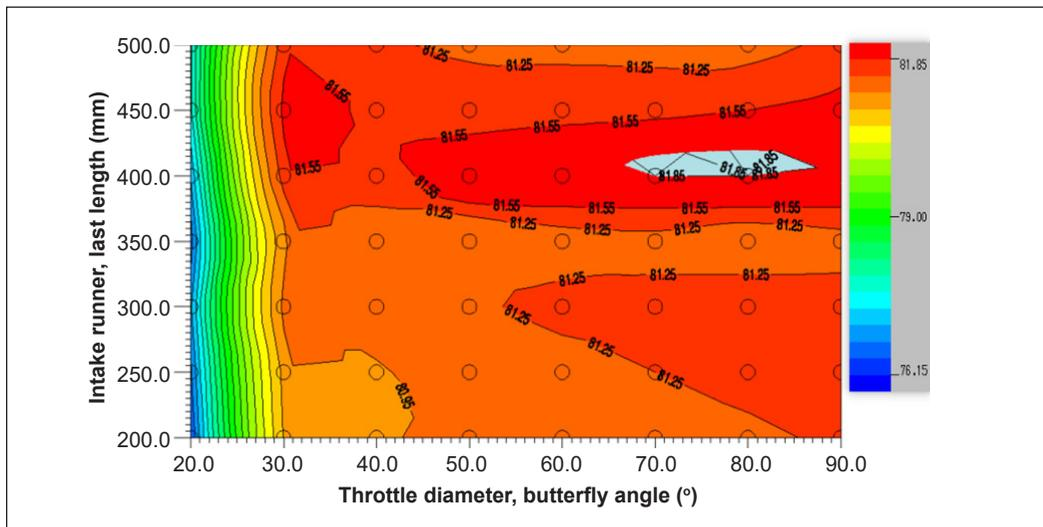
Figure 4. Volumetric efficiency at 1000 rpm
