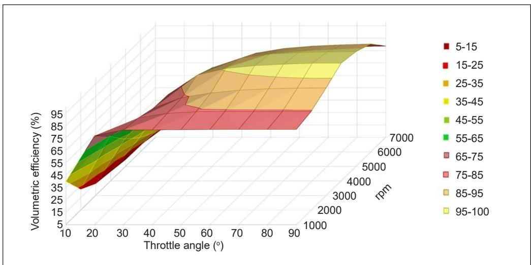
Figure 3. Volumetric efficiency mapping at different throttle angles across a range of rpm
