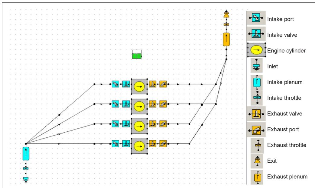
Figure 1. Configuration of simulation in Lotus Engine simulation
